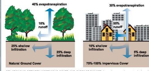
**RELATIONSHIP BETWEEN IMPERVIOUS COVER AND SURFACE RUNOFF.** Impervious cover in a watershed results in increased surface runoff. As little as 10 percent impervious cover in a watershed can result in stream degradation.
